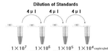
To generate a standard curve on the real-time system, all four dilution standards should be used and defined as standard with specification of the corresponding concentrations.
