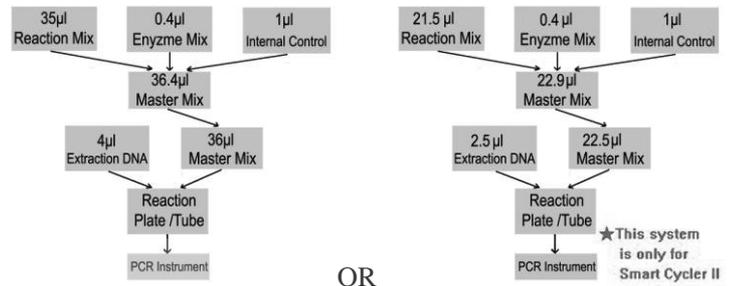
※PCR system without CY5 channel may be treated with 1µl Molecular Grade Water instead of 1µl IC.
